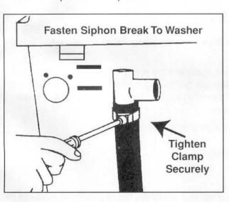
3. Install the end of the hose which was cut off over the other open end of the siphon break. Slip the open end clamp over the hose where it fits onto the siphon break. Using the screw provided, secure the clamp to the washer. Use the hole provided in back panel.
