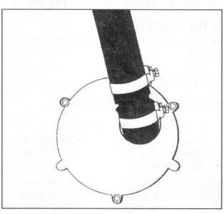
Install the gooseneck end of the drain hose into the standpipe. Be sure an airtight connection is **not** made between the drain hose and the standpipe.
